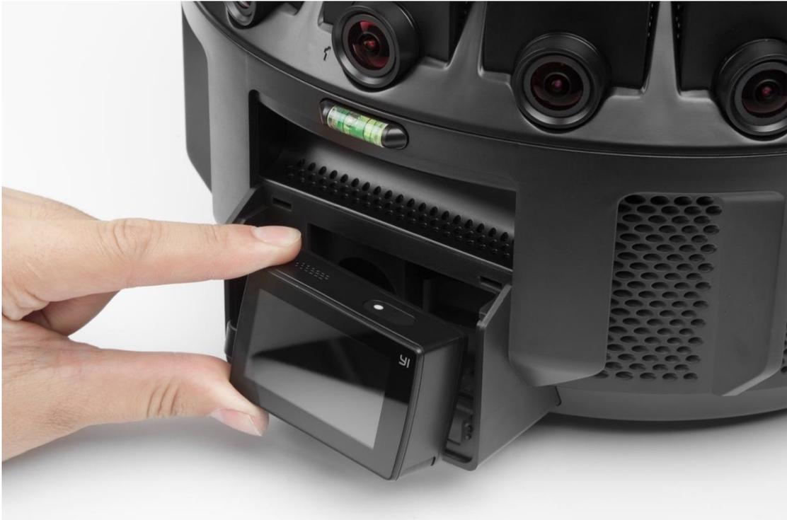
3. Align the new controller's lens with the inner frame, reconnect the USB cable, then push the new controller into the controller holder with the screen facing out.
