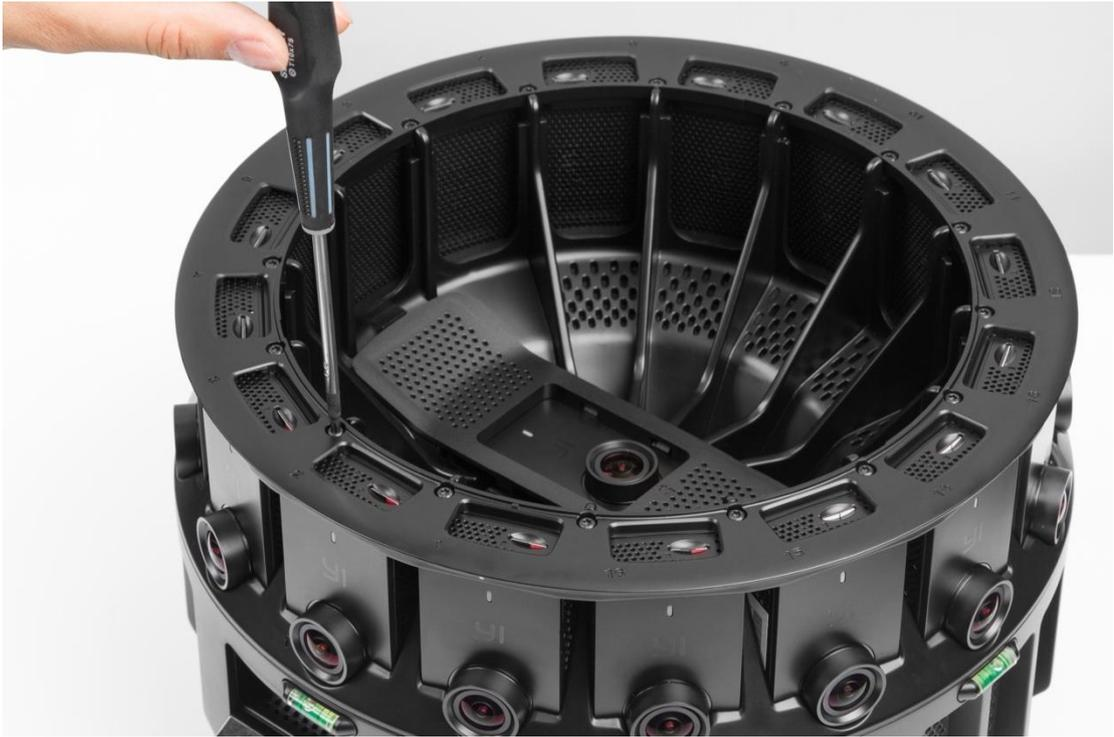
2. Pull out the problematic unit and insert the new one.
