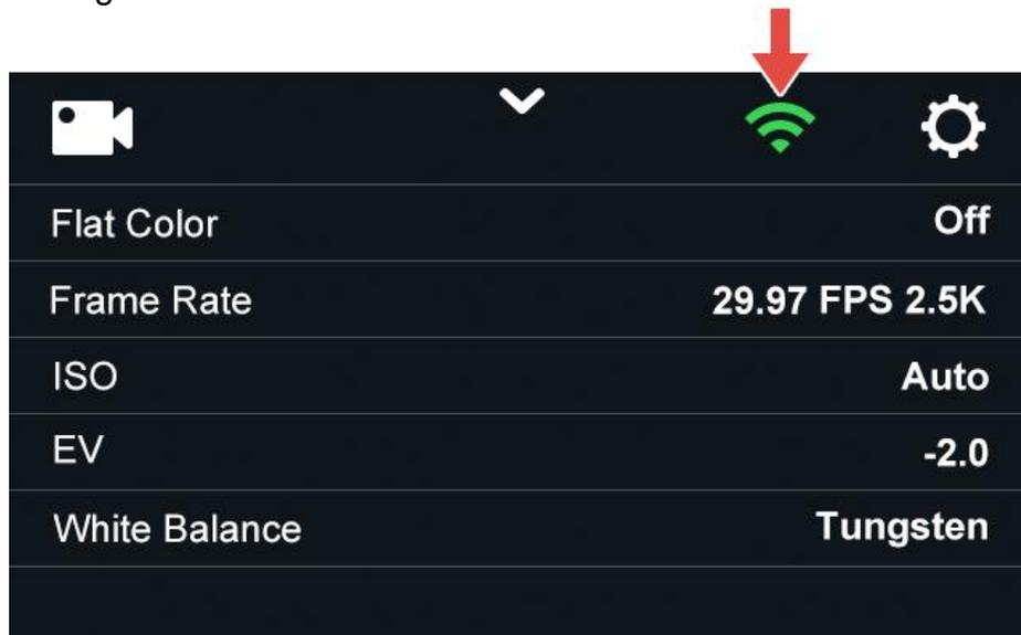
Tap the button to toggle Wi-Fi ON. The SSID and password are shown.
