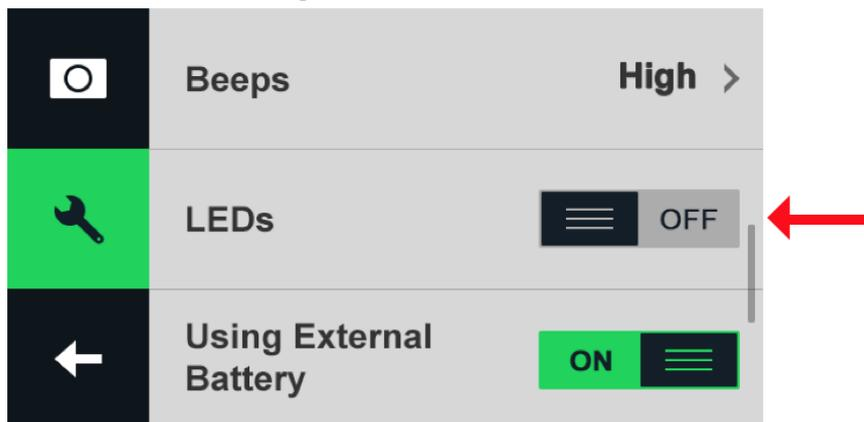
If the switch is on (default), when unit cameras are recording, the status lights will be red and flash. When unit cameras are free, the red status lights are on.
