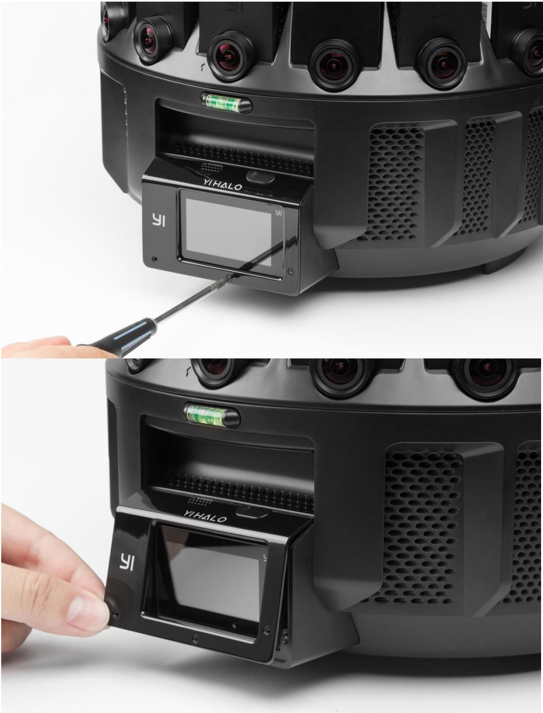
2. Disconnect the controller from the USB cable, then remove the controller and set it aside.
