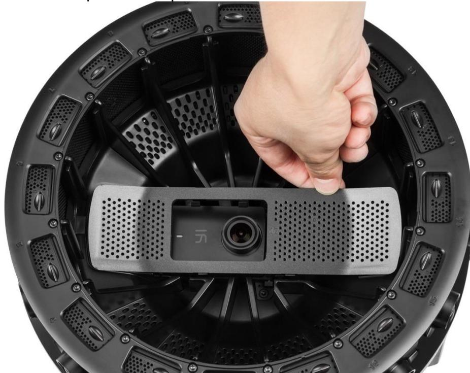
2. Pull the up camera out of the camera holder.
