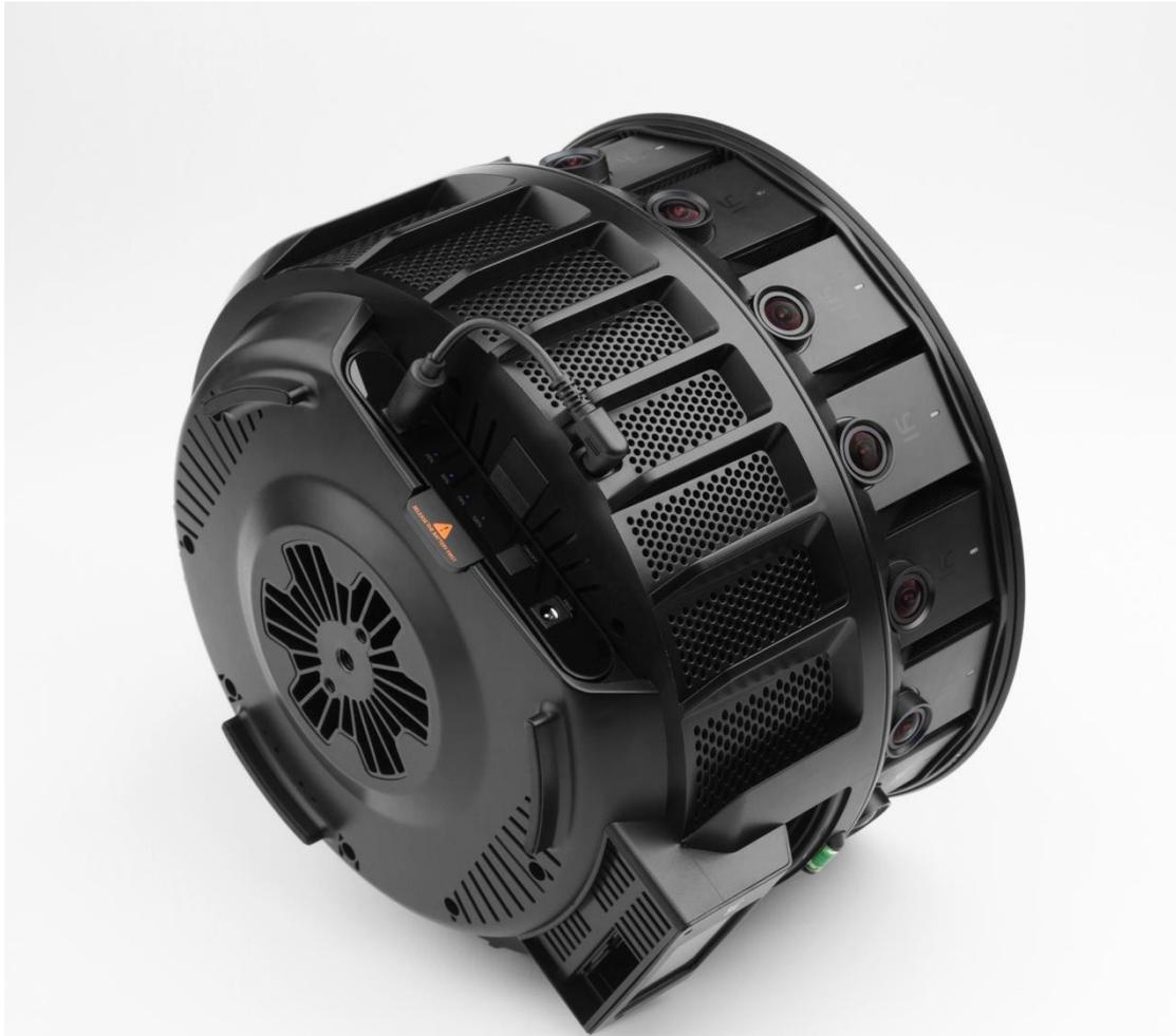
If you want to remove the battery, press the button at the bottom of the rig and pull the battery out.
